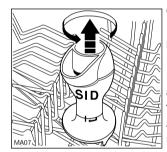
Check that the Super Intensity Dispenser (SID) is not clogged with detergent residue or soil. If necessary, rinse it under running water after having removed it from the basket by twisting it anticlockwise and pulling it upwards.
